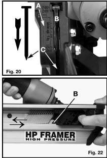
5. Pull the follower (B) Fig. 22, all the way to the rear of the magazine and release. The follower will apply pressure to the strip of nails to feed it into the driving mechanism.
